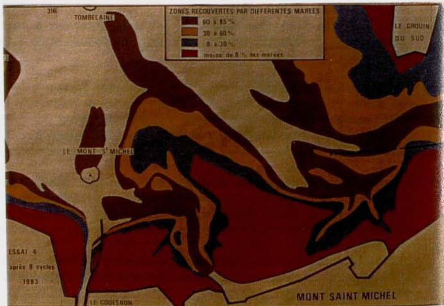
AVEC BARRAGE AMENAGE , DIGUE COUPEE,RESERVOIR EST
